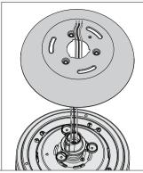
Thread the wires through the top housing. Place the top housing onto the motor housing so that the holes in the top housing lineup with the holes in the motor housing and the adapter.
