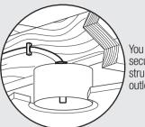
You must be able to secure the fan to building structure or fan-rated outlet box.
