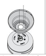
Place the canopy on the top housing. Ensure all four screw holes line up with the screw holes in both the top housing and the adapter.
