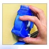
4. Cutting: Tip the applicator and press the metal cutting blade against the tape. Secure the roll of tape with your index finger as you cut.
