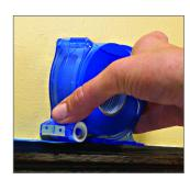
3. Keep the bottom of the applicator flat as you slide it along the trim. The rollers will press the tape down.
