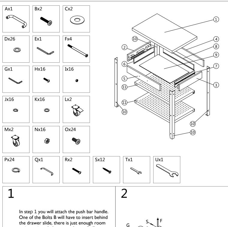
to insert it and please use the small allen wrench G to tighten the Bolt B with washers C & D into the push Bar A.
