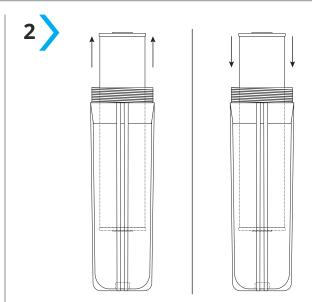
Remove the old filter and install the new filter. Ensure to center the filter cartridge properly in the housing.
