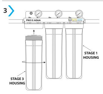
Inspect the O-Ring on the housing for any damage or cracks. Ensure the O-Ring is sitting properly in the groove. Lubricate the O-Ring and housing threads with silicone lubricant or a food-grade lubricant.
