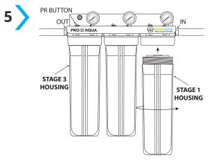
Install housing(s) onto the corresponding head and turn clockwise until snug.
