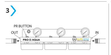
Attach your incoming supply line to the "IN" Port on the system then attach the line going into your home to the "OUT" port on the system.
