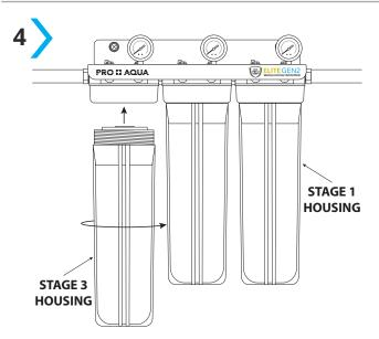
Reinstall the housing by pushing the housing up and at the same time turning the housing clockwise. Ensure to keep the housing and filter cartridge straight. Improper installation will cause the filter cartridge to not sit properly in the housing and will prevent the housing from closing all the way.
