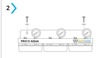
Install system to wall using the included SS bolts.
