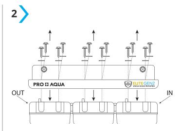
Remove the 12 bolts and washer to separate the Cap Module from the Bracket.
