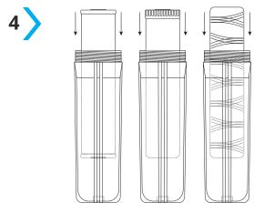
Unwrap cartridges and drop into the correct housings, centering on the stand pipe in the bottom of the housing. Stage 1 is closes to the "IN" port on the system.
