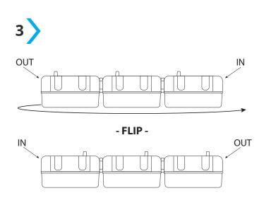
Flip the Cap Module so the IN port is on the opposite side.
