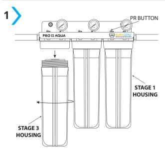
Remove housing using the housing wrench by turning the handle counterclockwise.
