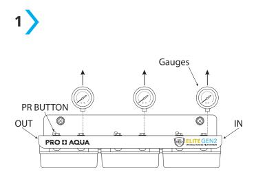
Carefully remove the Pressure Gauges from the system.
