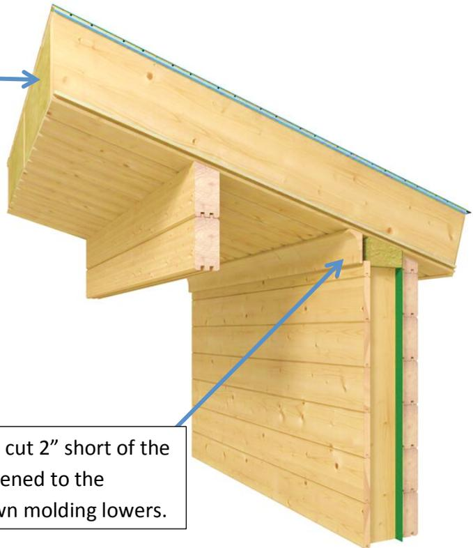
Interior wall cover boards must be cut 2" short of the ceiling and a crown molding is fastened to the ceiling. As the wall settles the crown molding lowers.
