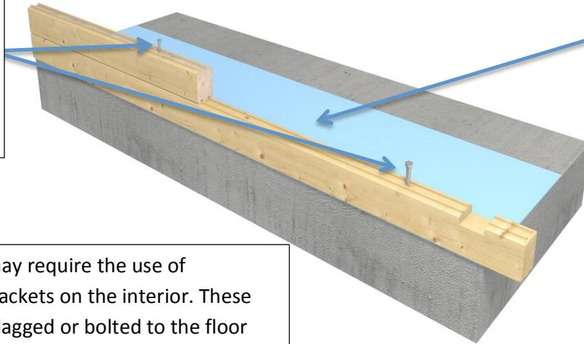
A moisture barrier can be applied between the first wall log and the surface it's being mounted to
