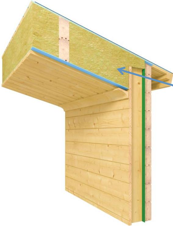
Insulating the ceiling can be done from the interior by placing insulation between the purlins and then applying a cover board to the underside of the purlins. Insulating from the underside reduces ceiling heights. Walls can be increased in height if requested.
