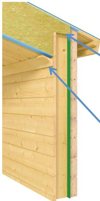
Studs are cut 2" short of ceiling height to accommodate shrinkage.
