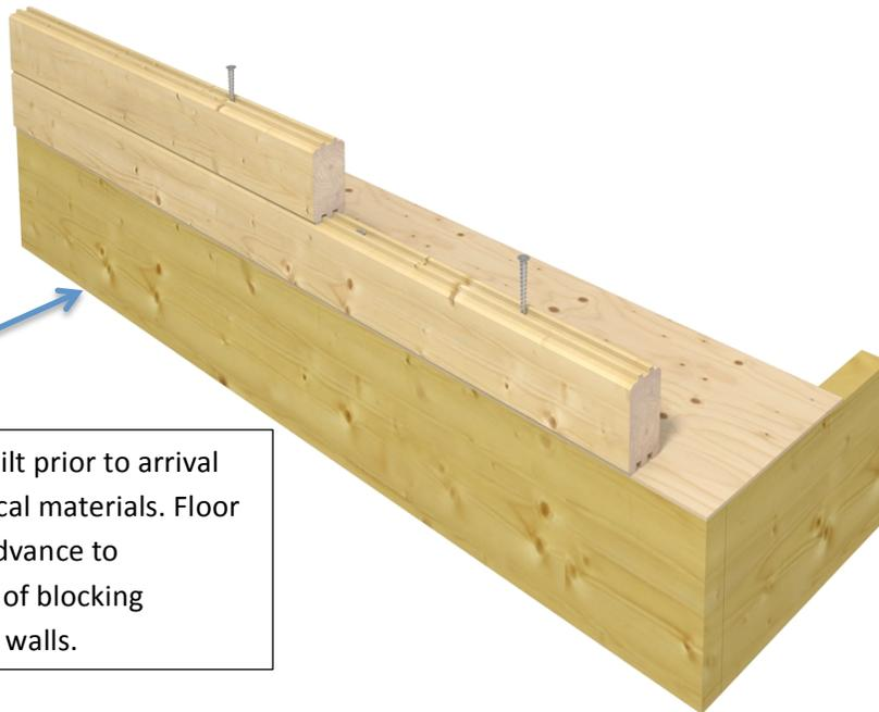
Wood sub floors are built prior to arrival of the package using local materials. Floor plans are provided in advance to determine the location of blocking required under interior walls.
