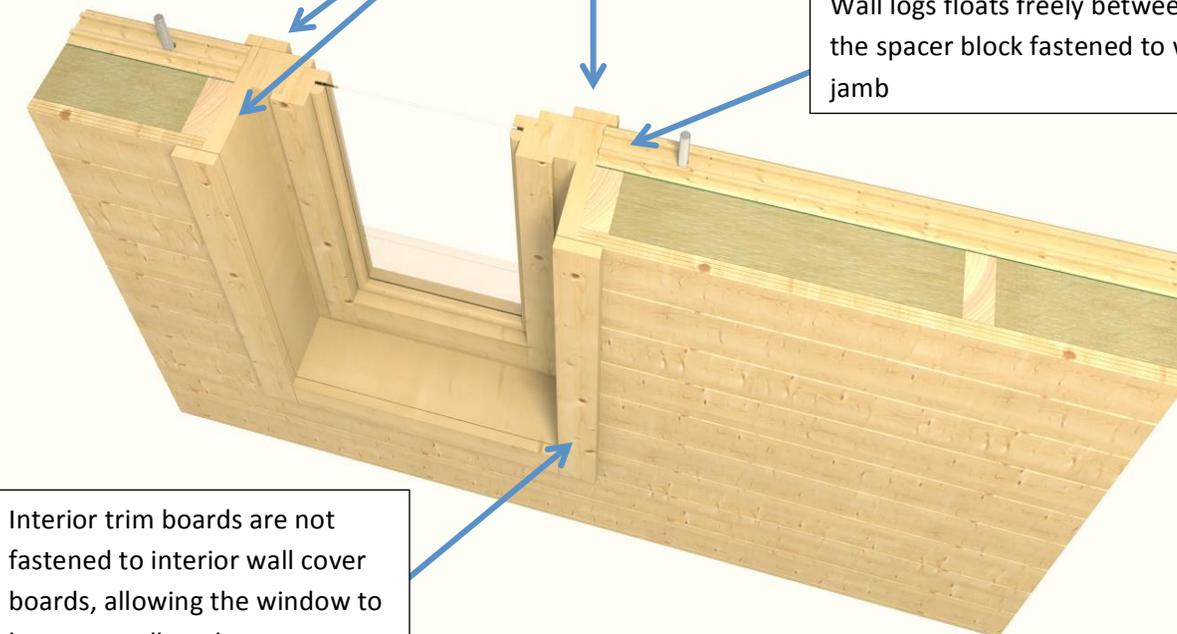
Interior trim boards are not fastened to interior wall cover boards, allowing the window to lower as wall settles.
