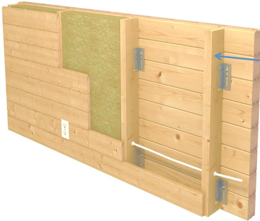
Studs with a depth required for the insulation being used, are installed 16" or 24" on center. Metal brackets are provided to attach the studs to the wall logs. No top plate or bottom plate is required. The metal brackets are designed to allow the exterior wall logs to settle while the studs remain stationary
