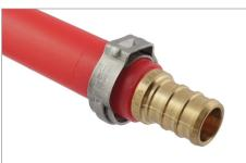
2. Slip PEX pinch clamp over tubing and insert fitting. Place pinch clamp 1/8" below edge of tubing.
