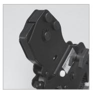
1. Ratchet the Pinch Tool to the closed position until the LED light comes on.
