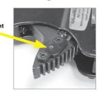
2. The battery compartment has a plastic cover attached with two screws.
