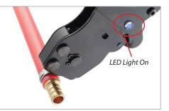
3. Place pinch clamp nub between tool jaws and ratchet the clamp (approximately seven times) until the LEDlight comes on. This will assure that the pinch clamp is fully engaged.
