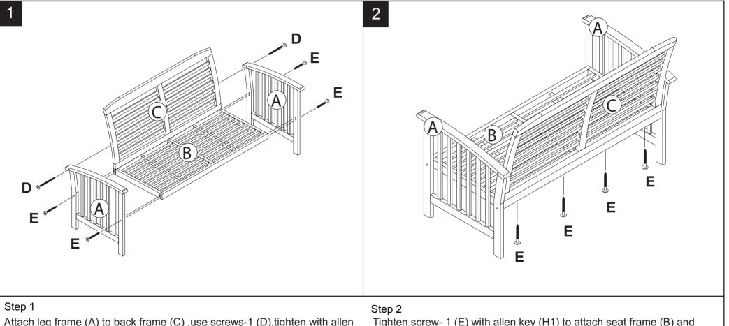
Attach leg frame (A) to back frame (C) ,use screws-1 (D),tighten with allen key(H1).Use screw -1 (E) to connect leg frame (A) with seat frame (B), tighten with allen key (H1).
