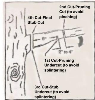
Make third cut as close to tree trunk as possible on underside of limb stub. Use top of guide bar to make this cut. Cut 1/3 through diameter of stub.
