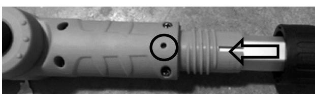
5. Tighten the shaft coupling B by turning it clockwise.
