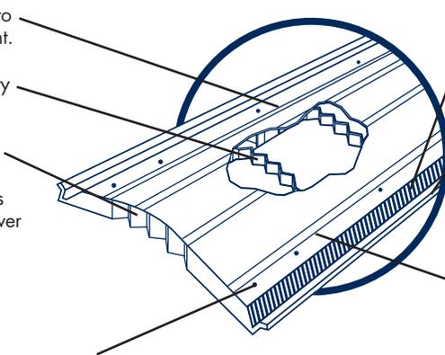
**18 Square Inches Net Free Area.** Plus an external baffle to enhance airflow makes VenturiVent Plus a superbly effective product for attic ventilation.
