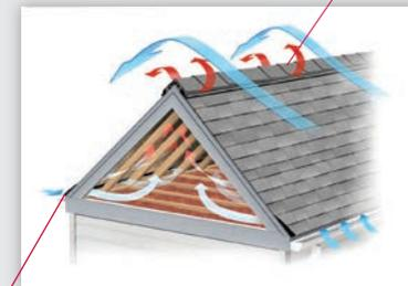
*Air enters attic through intake vents low at roof's edge or in the soffit/eaves.*
