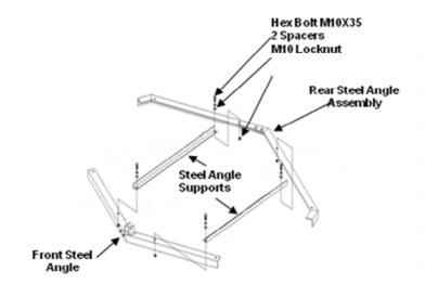
Step 4 Connect the Front Steel Angle Assembly to the Rear Steel Angle Assembly with the two Steel Connecting Straps using the Hex Bolt and Lock Nut. (4 Places)
