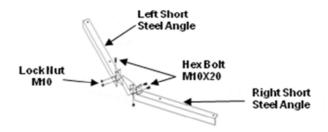
Connect the Front Steel Angle Assembly to the Rear Steel **Step 3** Angle
