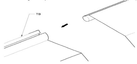
**STEP 7:** Pull the remainder of fabric over the fame with the valance hanging down below the (NC) and (FB) bars.
