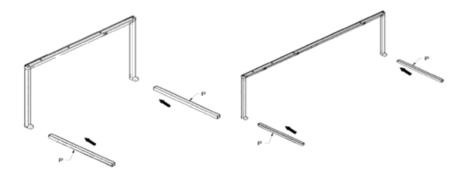
Step 4: Connect the Front Bar (FB) tot eh projection Bars (P). Velcro will be facing out. Secure with Self tapping screws.
