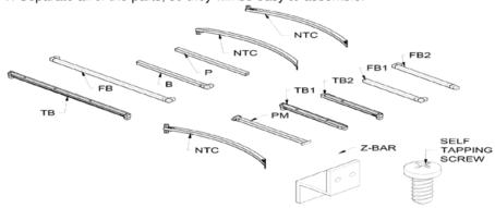
**Step 2:** Connect Top Bar (TB) to the (2) two back bars (B). Make sure the C-Channel is towards the back. The Velcro on the back bars should be facing the rear. Use a rubber mallet to fully seat the tubing into the fitting. Secure with self-tapping screws.
