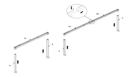
Step 3: Connect Both Projection Bars (P) in the other ends of the Back Bars (B). The Velcro will face outwards.
