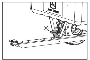
1. Lock cart foot pedal (H) in place & park machine safely. (See Parking in the Safety section).
