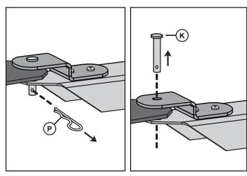
1. Remove spring locking pin (P) and clevis pin (K).
