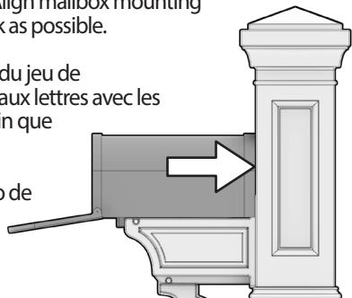
**TIP:** Feed bolt (H1) through mailbox and slot in part 'C'. Then, put lock nut (H3) in socket and balance washer (H2) on top.
