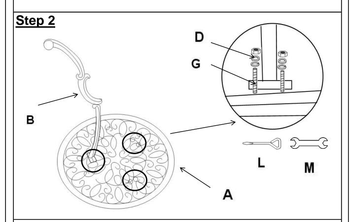
Lay the Table Top(A), Top being floor facing, onto a flat soft clean surface .
