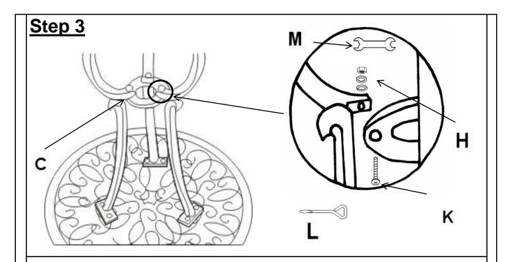
Attach the Leg Ring Support Ring(C)to Table Legs(B) using Bolts(K), Washers, Spring Washers, and Nuts (H).
