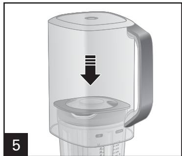
5 Place quiet shield over blender jar assembly.
