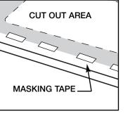
Drop in side: 1. Select the drop-in kitchen sink template that applies to the model sink you are installing. Cut out the inside of the template and discard the cutout portion. Locate the template front to rear and right to left on the countertop so the bowl will not interfere with the cabinets below. Attach the template to the countertop with masking tape and draw a pencil line around the inside of the template. Discard the template.
