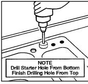
4. Identify fixture hole locations. Drill a starter hole from reverse side. Working from the top side as illustrated, position a hole saw on the starter hole and drill to complete the fixture hole. Attach faucet, drain, and accessories according to manufacturer's instructions.
