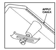
5. For final fit, apply a bead of caulk (not included) to the underside of the sink flange and position sink into countertop opening. First, tighten screws in front, then tighten rear screws.
