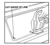
3. Using a saber saw, cut inside of cutout line. Trial fit sink to check proper fit.
