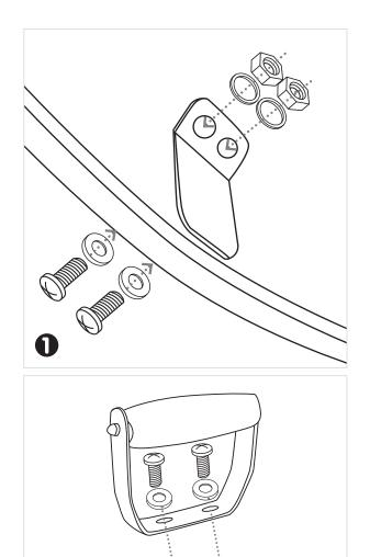
Align holes in Connecting Brackets • with the Screens and the Screen Door •. (*Note: Connecting brackets should be placed on INSIDE of screens*). Slide M6x18 Washer • onto M6x15 Screw • and through the hole in the Connecting Bracket and Screen. Secure with M6x9 lock Washer • and M6x15 Nut •. Repeat with remaining Connecting Brackets.
