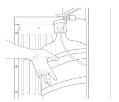
7. If you are using a 3 gallon bottle rather than a 5 gallon bottle you can adjust probe by pressing the two tabs at the head of the probe and sliding the collar down to the neck of the bottle.
