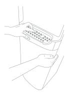
3. Gently pull the drip tray toward you to release it. Once it has been released you can remove the drip tray from the door of the cooler to empty it.
