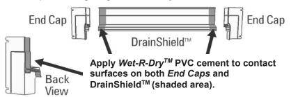
Slide End Caps fully in place. Wipe excess PVC cement. Hold glued parts for 1 min for PVC cement to dry.
