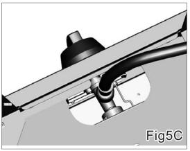
**Step 4**: Place the Wind Shield as shown–But, do <u>not</u> fasten in place.
