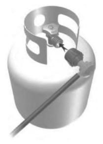
Cylinders must be filled before initial use. All handling, transport, filling and storage of LP gas cylinders must be in accordance with NFPA 58 Storage and Handling of Liquid Petroleum Gases, or CSAB 149.1 Natural Gas and Propane Installation Code. Cylinders must be suitably tied down during transport. Do not place any other items on top of cylinders at any time. Cylinders are not to be exposed to excessive temperatures or high heat.
