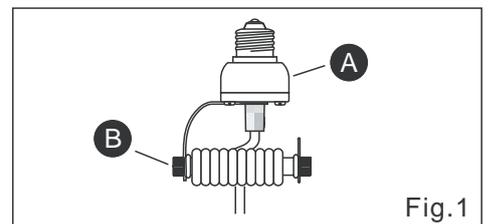
2. Screw the adapter (A) into the light bulb socket in your recessed light fixture.
