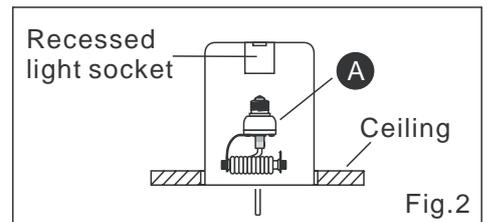
3. After finger loosening the compression nut (D) by turning it counter-clockwise, slide the canopy (C) up the cord and against the ceiling.
