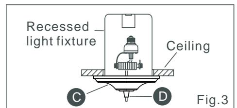
4. To hold the canopy in place against the ceiling, finger tighten the compression nut (D) by turning it clockwise.
