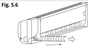
3. Now, you will need to lightly tape the refrigerant piping and drain pipe together in a bundle, using electrical tape, making sure that the drain pipe is at the bottom. <u>DO NOT</u> tape the ends of the piping (connectors). Refer to Fig 5.7 and the image below for the correct orientation of the piping when taping.
