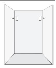
To insure a proper installation, it will be necessary to affix wall cleats to the closet side walls. These are typically 5" x 12" x 1/2" blocks of wood which are attached to the wall using screws and drywall anchors. Attach the pole socket to the cleat to allow 2-1/2" of space between the pole and a shelf above the cleat.
