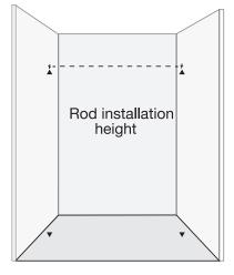
Next, determine the installation height of your rod. Allow sufficient height to insure your clothing hangs freely. Mark the position on each wall for pole sockets.
