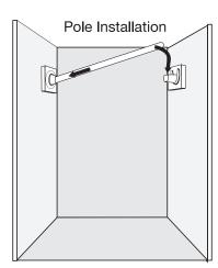
Insert one end of the closet pole into the enclosed pole socket. Once the pole end is fully inserted, place the other end in the opposite pole socket. Check to make sure pole is level and secure. Installation is complete.
