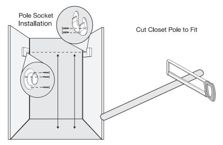
Once the cleats are firmly attached, screw in the pole sockets using the included screws. It may be necessary to pre-drill pilot holes. Make sure the sockets are level with each other across closet pole span.
