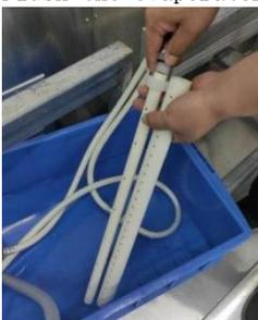
Rinse the sprinkler pipe and core rod
