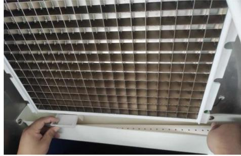
8. While soaking the parts, use a nylon brush or soft cloth dipped in cleaning fluid to wipe the surface of the parts that are in contact with water and ice, such as evaporator ice trays, ice shields, ice storage buckets, etc. The damp cloth wrapped disposable chopsticks to clean up). Then rinse with clean water (rinse 5 times).
