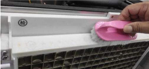
Brush the plastic parts around the evaporator
