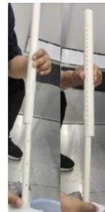
■ **Disassembly and assembly of the water baffle:** grasp the middle position of the water baffle, use a flat-head screwdriver to apply force from one side to the other, until one side of the water baffle comes out of the pin hole.
