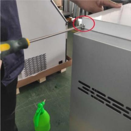
Lift the top cover slightly upwards first, and then gently pull back to pull out the top cover
