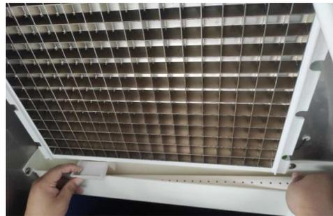
While soaking the parts, use a spray can to evenly and completely spray the disinfectant on the surface of the parts that are in contact with the ice, such as the evaporator ice tray, ice shield, ice storage bucket, etc. (the dead corners can be wetted with disinfectant Disposable chopsticks wrapped in a rag to
