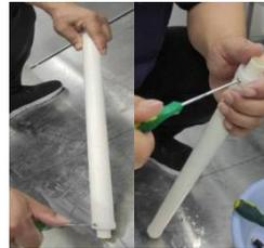
Unscrew the plastic cover and take out the plastic core rod
