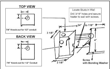
Heaters are not to be mounted closer than 2-1/2" inches from ceiling. 4" inches or more is recommended for max performance. Do not install less than 6 ft. above floor and 2-1/2 inches from ceiling and 1 inch above top of any fabric.
