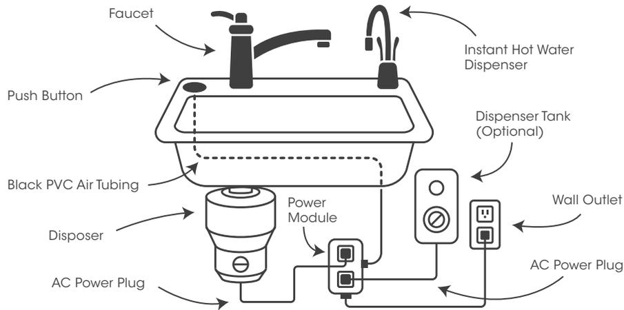
**1) Positioning the push button switch.** Remove LARGE plastic nut from the air switch main threads and insert into existing standard sink hole leaving the gasket above the sink/counter. If a hole does NOT exist, drill a 1 1/4" diameter hole into the counter where you want the button to go.
