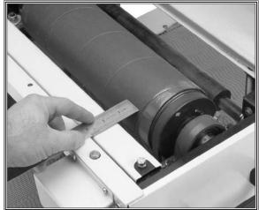
Figure 31. Measuring drum alignment.
