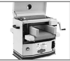
Figure 38. Gauge boards in position.
