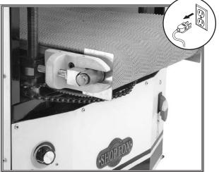
Figure 51. Conveyor belt loosened at the front adjustment bolts.
