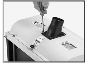
Figure 8. Dust port installation.
