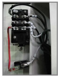
Figure 67. ON/OFF switch wiring.
