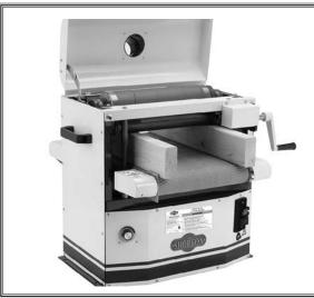
Figure 28. Gauge boards in position.
