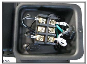
Figure 64. Drum motor wiring.
