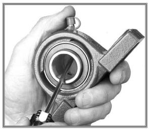
Figure 59. Bearing positioning for removal.
