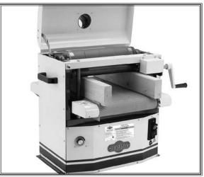
Figure 34. Gauge boards in position.
