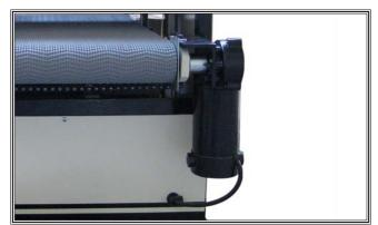
Figure 63. Feed motor.
