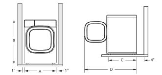
Install the washing machine on a solid floor that is strong and rigid enough to support the weight of the washing machine, even when fully loaded, without flexing or bouncing. If the floor has too much flex, you may need to reinforce it to make it more rigid. If the floor is not solid, it may cause severe vibration and noise.
