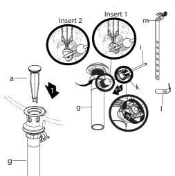
Insert waste stopper (a) into drain flange. Remove extender rod (m) and clip (l) from drain off pole (i). Reomve nut (k). Insert drain off pole (i) into drain pole opening of tailpipe (g). See insert 1. Secure nut (k) to drain off pole opening of tailpipe (g).
