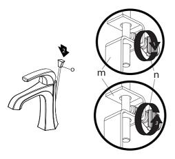
Loosen thumb screw (n) on extender rod (m). Push down on lift rod (o) until stopper is in open position. Retighten thumb screw (n).
