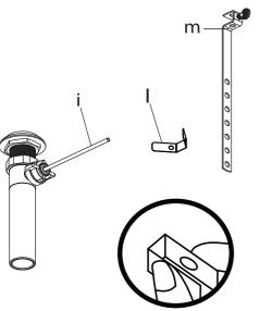
Attach drain off pole (i) to extender rod (m) with clip (l).
