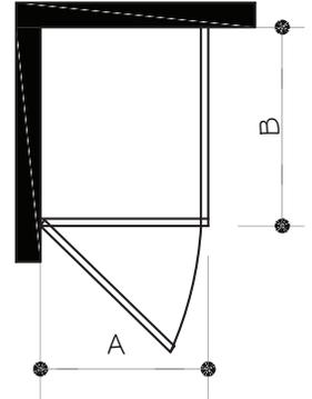
A & B DIMENSIONS WERE MEASURED AFTER SHOWER ENCLOSURE WAS COMPLETELY INSTALLED
