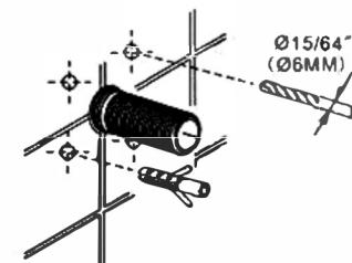
4、Drill holes by an electric drill in the
