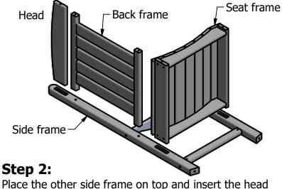
and seat frame into the pockets. Also, line up the back frame
