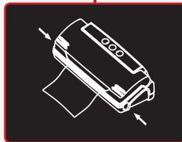
**Step 3:** Once the Sealing Indicator Light is no longer lit, press the Cover Unlock Buttons to unlock the top cover.
