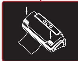
**Step 2:** Press the cover down **firmly** on each corner of the top cover until it locks into place with an audible click. To seal, press the **"Seal Button"**. To vacuum and seal, press the **"Vacuum & Seal"** Button.
