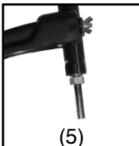
1. Unscrew knob and remove the entire trimmer head assembly. A pair of pliers may be needed to remove the lock washer from the spool housing.
