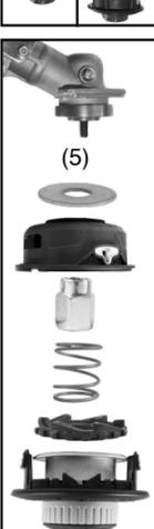
1. Unscrew the knob and remove the entire trimmer head assembly. Unscrew the shaft extension to expose the primary shaft.
