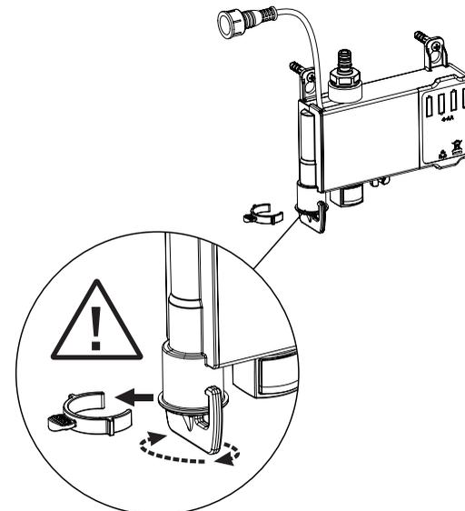
Switch to manual operation when the power is low or the sensor is out of order.
