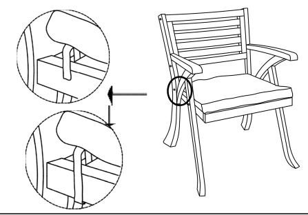
Inspect the Chair and make sure all parts are adequately connected. Place Seat Cushion(C) on to the seat of the Chair using the velcro straps as shown above.
