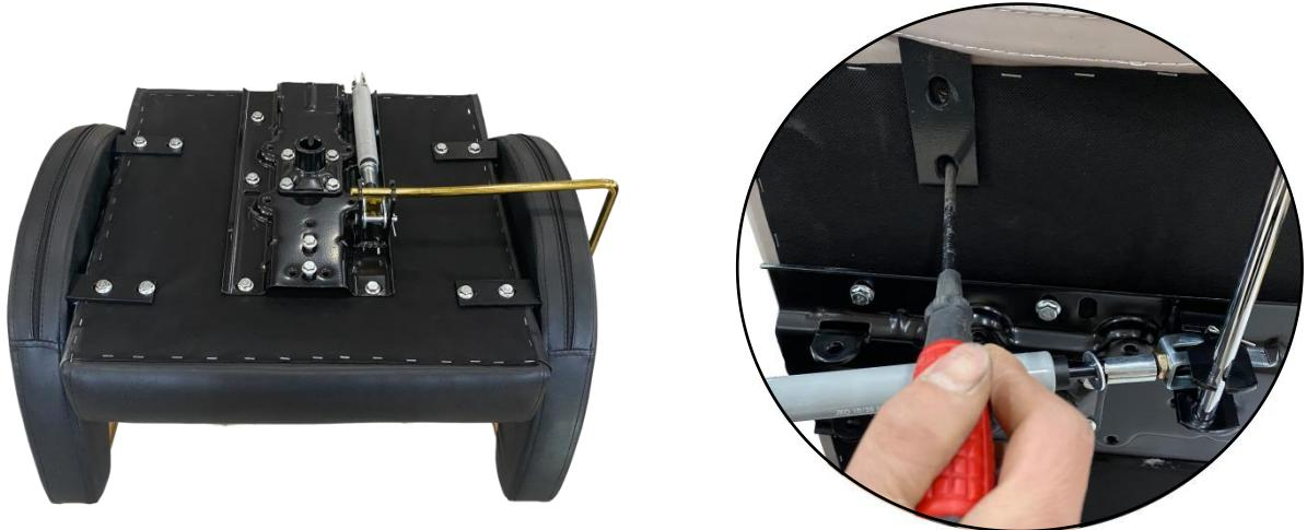
**Use a screwdriver to align the holes when you felt it's hard to assemble.**
