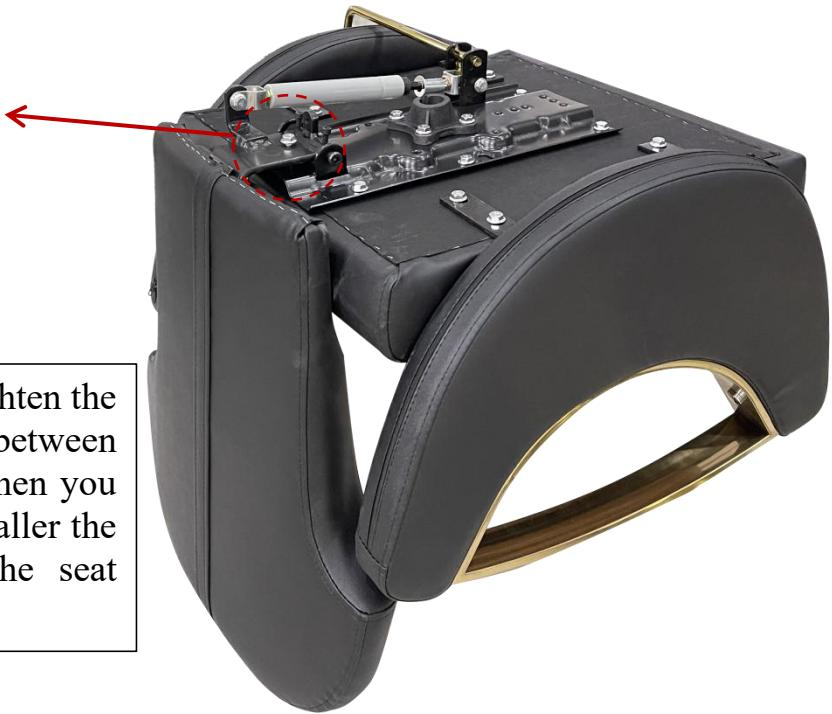
Please notice that the more you tighten the screw in, the greater the Angle between the back and the seat cushion; When you loosen this screw outward, the smaller the Angle between the back and the seat cushion (closer to 90 degrees).
