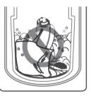
• Do not load bulky items such as pet beds that are too large or stiff to move easily around the agitator. Impeding the motion of the drum or agitator could cause damage to the items or the washer.
