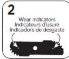
This blade has wear indicators (Fig. 2). When blade wears to the small hole at each end of the blade it will give approx. 3/8 in (9.5 mm) depth of cut and should be replaced.
