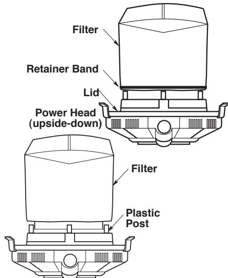
**IMPORTANT:** To avoid damage to the blower wheel and motor, always reinstall the filter before using the vac for dry material pick-up.
