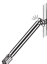
Bend plastic straps back and forth until they snap off, leaving plastic ring in place.
