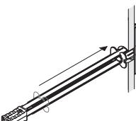
Slide plastic ring along straps until flange of ring is flush against wall.
