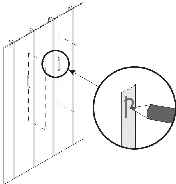
**2** Decide where to locate the top of the vertical panel. Mark a hang line for the rail 8.5" down from the top of the vertical panel.
