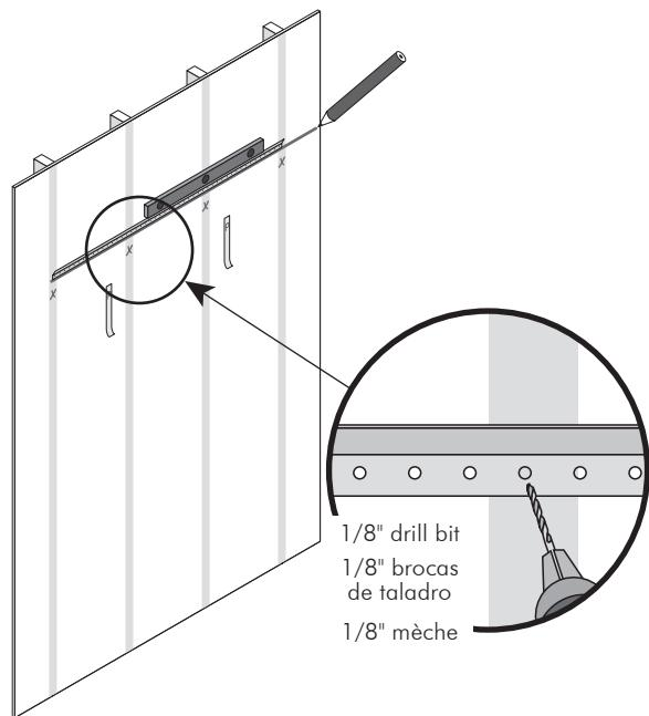
**6** **IMPORTANT.** If a vertical will be more than 3" from a stud, you'll need to use a toggle to support that panel. Mark toggle locations next to vertical panel locations. If panel will be less than 3" away, skip to Step 9.
