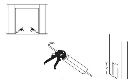
Silver Line strongly recommends that you use a membrane or vinylbased sill pan to ensure a weathertight seal. Follow the sill pan manufacturer's installation instructions.
