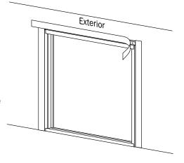
IMPORTANT – To create a weathertight seal, ensure that the flashing fully covers the entire length of the jambs and head of the door around the door opening. Pay special attention to the corners to ensure that there are no gaps in the flashing.
