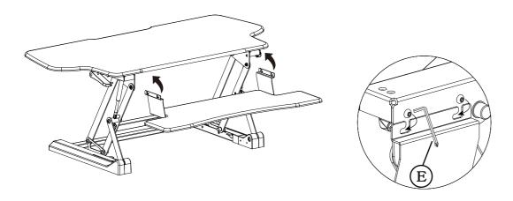
**STEP 5.** Pull up on both AIRLIFT® levers and top to lift.
