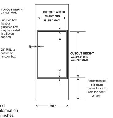
ATTENTION INSTALLER: All electric wall ovens must be hard-wired (direct-wired) into an approved junction box. A plug and receptacle is NOT permitted on these products.
