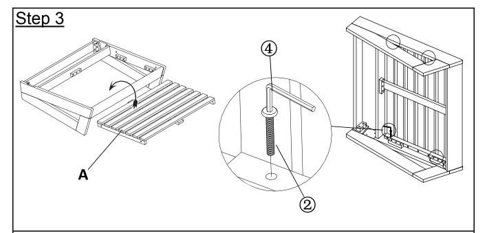
Insert Seat Panel (A) into assembled on step 2 using Bolts (2) with Allen key (4) as shown in picture above.
