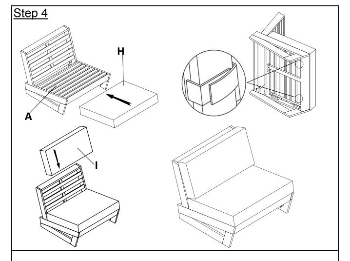
Place Seat Cushion(H) and Back Cushion(I) onto the Chair, turn the Chair down and tie the velcro straps of the Cushion (H) to the Seat Panel (A) as shown above Then EXERT pressure, floorwards onto the Chair with both hands.
