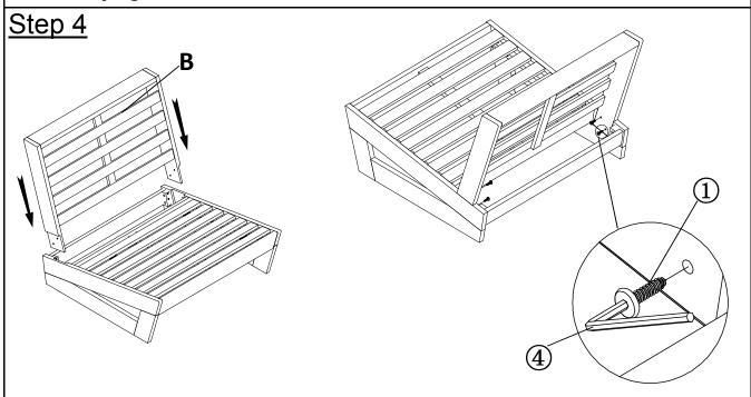
Insert Backrest Panel (B) to assemble of step 3 using Screws (1) with Allen Key(4) as shown in picture above.
