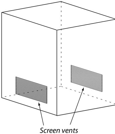
Make sure each opening has a total free area of not less than  $\frac{1}{2}$  square inch per pound (3.2 sq. cm/kg) of stored fuel capacity and not less than a total free area of 10 square inches (64.5 sq. cm).
