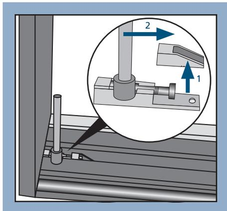
3. Slide the pin assembly back into the base and snap the top cover back on and fasten through the remaining hole with the other screw.
