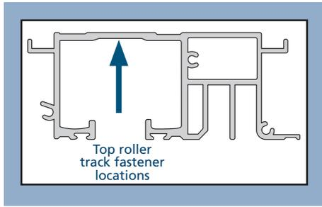
2. Secure the top roller track to the header using the provided #12 x 3" flat head screws through the pre-drilled holes.
