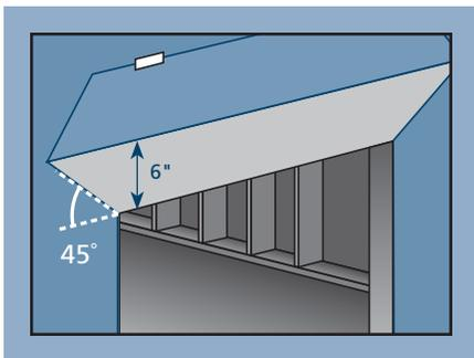
3. Trim the sides sufficiently to allow the nailing fin to be mounted against the sheathing.
