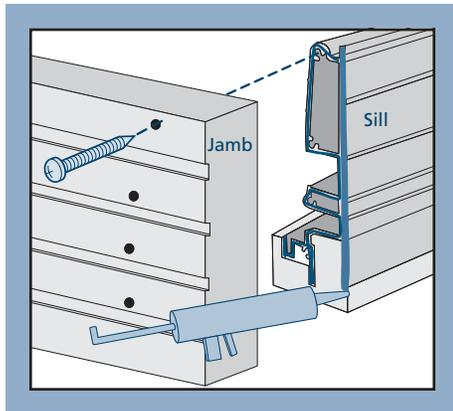
3. Clamp the frame corners as needed to ensure that the frame sections fit together flush and secure through the pre-drilled holes in the jambs with the provided #10 x 2-1/2" flat head screws.
