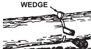
If you're unsure how a log actually lies, and how it will bend, change its lie. If too heavy to move without strain on the back muscles, use a lever bar such as a cant hook to move or roll it. **NOTE:** You may have need to use this procedure to free the saw, if you misjudged the position of the log.
