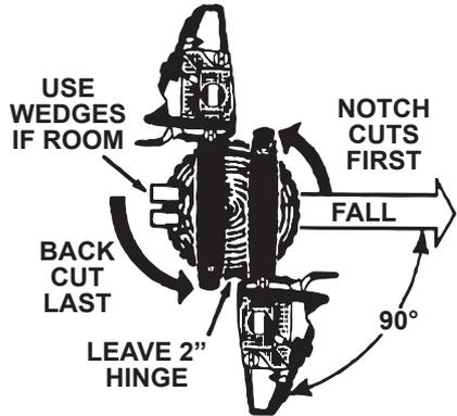
**⚠ WARNING! DO NOT CUT THROUGH THE HINGE! THE TREE CAN FALL THE WRONG WAY AND CAUSE PROPERTY DAMAGE, SERIOUS OR FATAL INJURY.**
