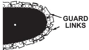
The low-kickback saw chain on your saw has depth gauges and guard links to reduce kickback. Depth gauges control the depth of cut. The guard links help to prevent the cutters from digging in too deeply at the bar nose. Low-kickback chain tends to resist penetration of the bar tip, which is the cause of kickback; however, the chain may "skate" along the surface of the wood. Skating the nose bar into an obstruction could result in a kickback.
