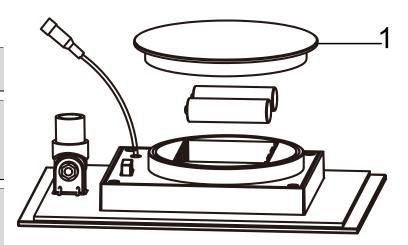
1. Twist off the battery cover, remove the old batteries and clean the battery contacts on the new batteries and solar lights. Replace with new 18500 Lithium 1000mAh rechargeable batteries and replace the battery cover (1).
