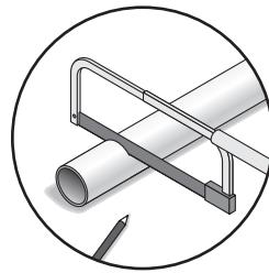
Cut rods to correct length with a hacksaw, if necessary.
