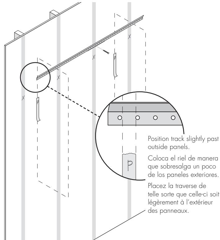
**5** Level the track and mark a line along its bottom edge. Drill  $\frac{1}{8}$ " pilot holes into each stud location and in the last hole of the track on both ends of the wall.
